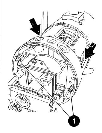
ASSEMBLING STARTING-MOTOR SOLENOID WITH CONTROL RELAY
